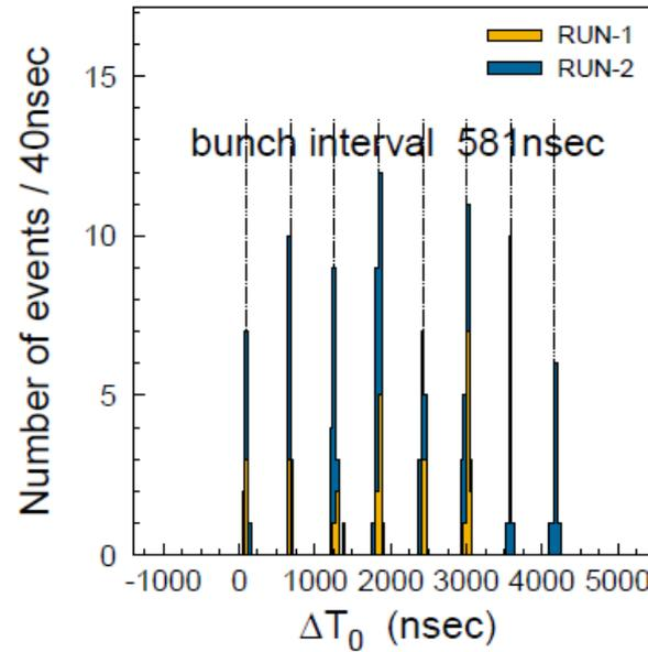
$$\Delta T_0 = T_{\text{GPS@SK}} - T_{\text{GPS@J-PARC}} - \text{TOF}(\sim 985 \mu\text{sec})$$
