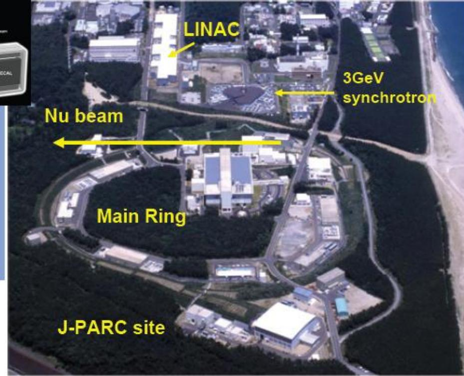
High intensity muon neutrino ( $\nu_\mu$ ) beam from the J-PARC 30 GeV proton accelerator to the Super-K detector 295 km away
